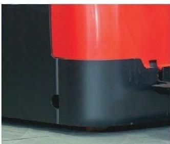
► The use of apron with 8 mm thickness allows to ensure the robustness of chassis and its strength even in case of collision against objects. The strong battery cover made out of steel helps to provide a high level of strength for this part.
