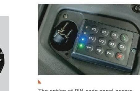
► The option of PIN-code panel access, which works not only with PIN-code but also with access cards (RFID), can significantly simplify the procedure of access limitation for the fleet which may be used by more than one operator.
